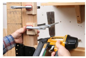
**Get ready for the gridwork.** I surrounded the gridwork with 1/4-in.-thick strips in front and behind it. The back ones go in first. I made these little L-shaped stops to help me place those strips right where I wanted them. Then I shot 18-gauge brads through the strips to lock them in. Thank goodness for air nailers.
