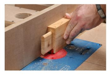
**Groove the rails too.** The middle and lower rails needed thae same grooves. I did that in two passes again on the router table, 1/4 in. at a time.
