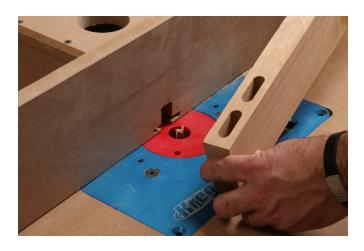
Grooving the stiles. The frame's long uprights needed 1/2-in. wide grooves, running between the lower mortises and the middle ones. I did that on the router table, making the grooves 1/2 in. deep in two passes.
