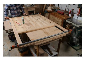
**Assemble in stages.** Start by slotting the boards into the lower and middle rail, with NO glue. Then apply glue to all of the mortises and tenons and you can add the top rail and side pieces (stiles). I used the bar clamps to draw the joints home, as they got pretty snug once glue was on them. BE SURE to use Titebond III, which is waterproof for outdoor use, and also gives you 10 or 15 minutes before it starts to cure and seize up.
