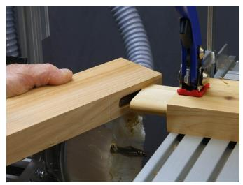
**It all starts with joinery.** I used 2-1/2-in. wide mortises and tenons in the two top rails, which are 3-1/2 in. wide. You want a snug fit that slides together with hand pressure, and the PantoRouter makes that easy.
