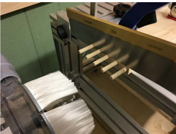
Cut the dowels free with a hand saw
