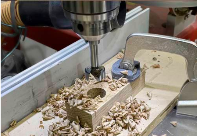
Drill a hole in a piece of scrap wood using a Forstner bit in your drill press
