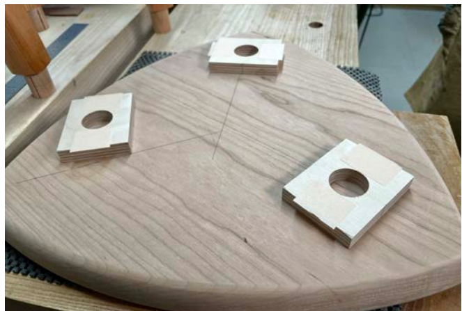
Locating round tenons on other parts such as the seat of this stool is simple. Using the Same Forstner bit from before, drill a hole in a scrap piece of wood and place some double-stick tape on the face.
