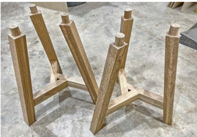
Once you have found the perfect fit, cut all of the tenons
