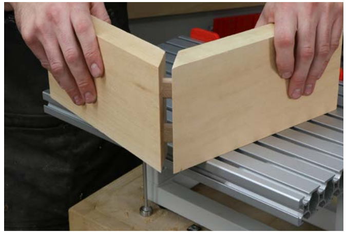
Double floating tenons in the angled workpiece on the PantoRouter® joinery machine took only a couple of minutes longer.
