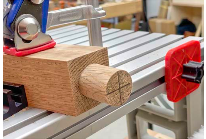
Cut the round tenon in the end of your workpiece starting high on the taper of the dowel template
