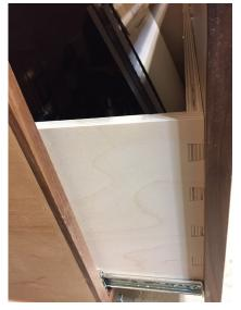
**Drawers courtesy of the PantoRouter.** McKnight used the machine to make the two upper drawer boxes, using finger joints, and the dovetails for the lower box. The drawer fronts are applied after the fact, by driving screws from inside the drawer boxes. This is a an easy, effective way to create a nice-looking cabinet of drawers, with even gaps all around the drawer fronts.
