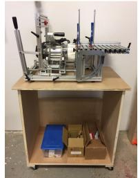
**Simple construction.** Screws and glue are a simple but effective way to build a plywood stand.
