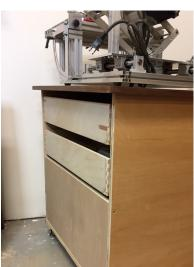
**Partial back.** A short panel in back is enough to stabilize the cabinet side to side, though you could run this panel to the top.
