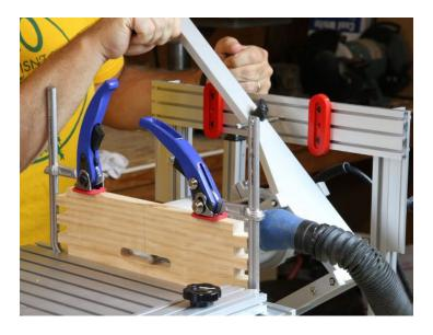
Handy handles, Panto-style. Use the tapered pointer, running it in one of the slots on the template holders, to rout a slot on the box ends, using the same 1/2-in. bit. Use the vertical mortising templates as stops, setting them 6 in. apart to create a 3-in.-long slot (remember the 2-to-1 pantograph ratio!).
