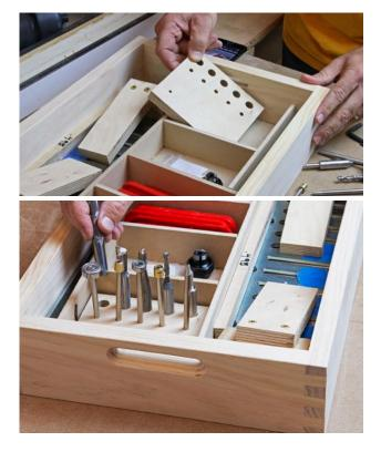
**Another PantoRouter trick.** When the box was done, I realized the handles were a bit uncomfortable as is, so I loaded a bearing-guided roundover bit in the PantoRouter, set the depth stop on the machine, and inserted the spinning bit into the handle slots, running it around the inner surface of the mortised handholds to create perfect roundovers.
