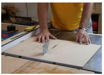
**Cut the bottom to size.** I determined its actual size by dry-fitting the box sides, taking inside measurements, and then adding the amount the box bottom sticks into its slots, minus 1/16 in. overall so it doesn't bottom out in the slots, preventing full assembly.
