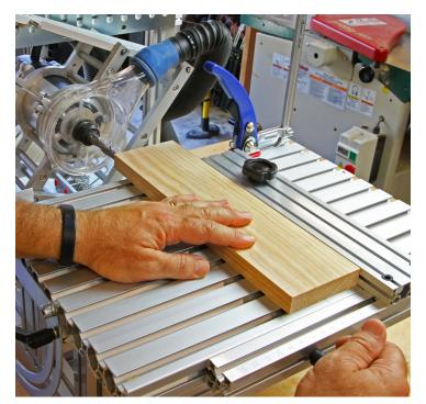
**Set the fence.** I recommend centering the workpieces, using the centering scale built into the fence. Then the fence can stay in that position, ensuring the joints go together cleanly no matter which way the workpieces are oriented.
